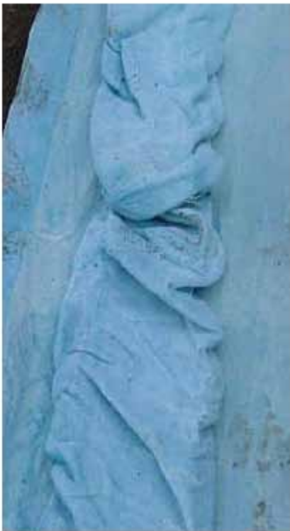
Figure 1 :: Example 1 of inner layer gathering up during impregnation.
