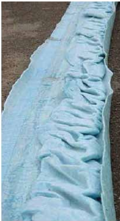
Figure 2 :: Example 2 of inner layer gathering up during impregnation.
